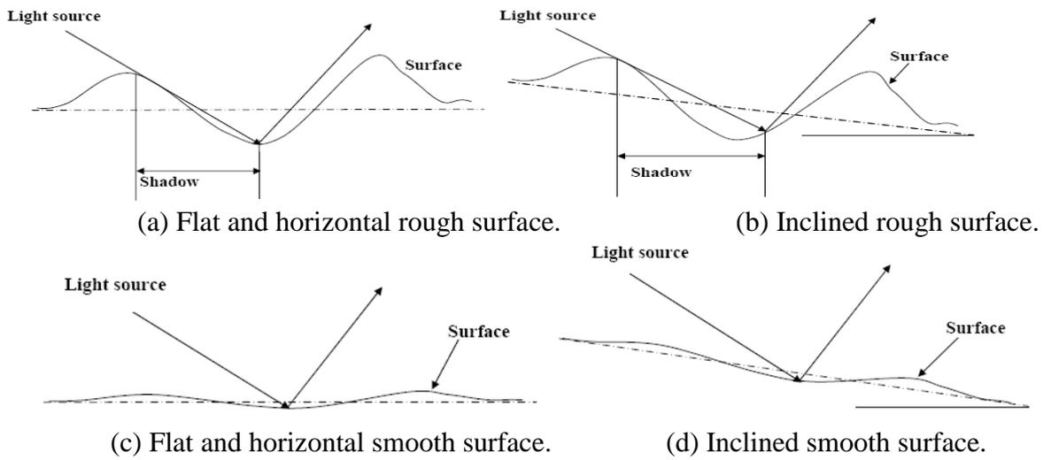
**Fig. 1** Illustration of creation of shadow on rough and smooth surfaces.
