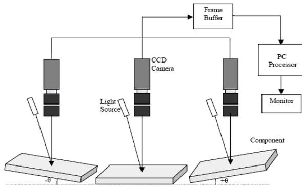
**Fig. 2** Schematic diagram of the machine vision system.
